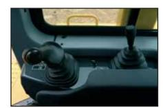
Blade and ripper control joystick
