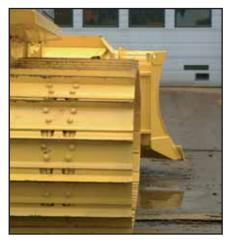
Unfolded blade (for operation)
