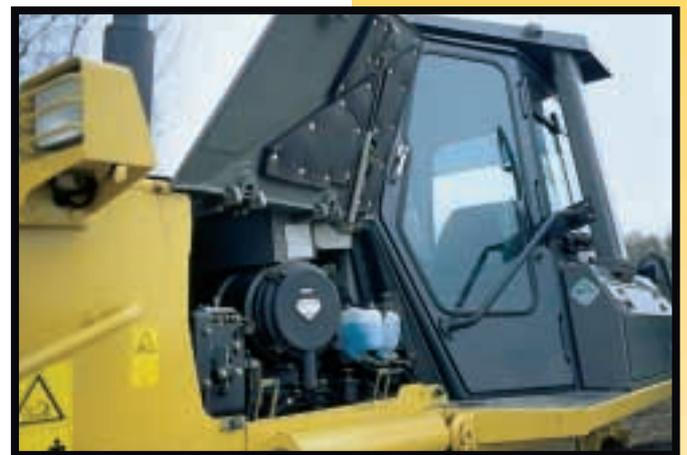
Gull-Wing Engine Side Covers with a gas-spring cylinder that opens widely, the engine and the auxiliary components can be checked easily.
