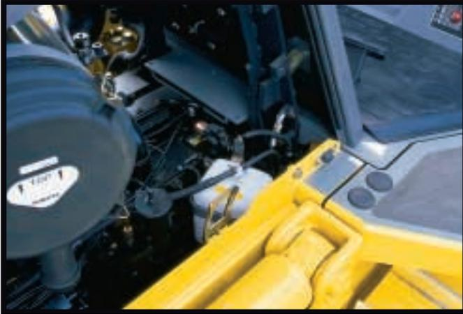
A radiator coolant reservoir makes it easier to check the coolant level and eliminates frequent refilling.
