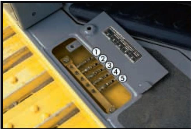
Centralized Oil Pressure Ports. The D61 offers the Komatsu exclusive centralized test ports on the right side of the chassis.
