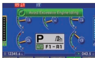
Eco-gauge, Eco guidance and fuel consumption gauge
