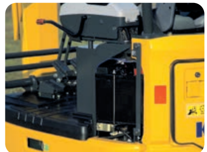
Left bonnet: easy access to the battery refilling
