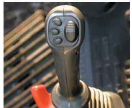
Joysticks with proportional control button for attachments
