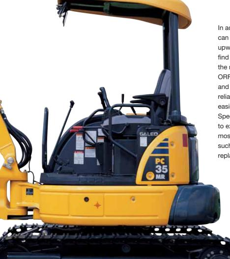
In addition, extra-ordinary maintenance can be performed by simply tilting the cab upwards: under the floor, the operator can find all major hydraulic components, like the main valve or the swing motor.
