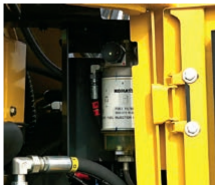
Fuel pre-filter with water separator
