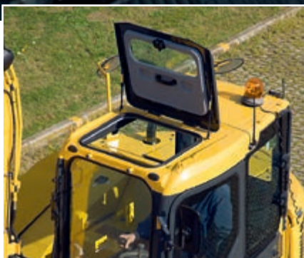
Opening skylight for overhead visibility
