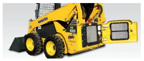
The hatchback: simple inspection and cleaning of the radiators
