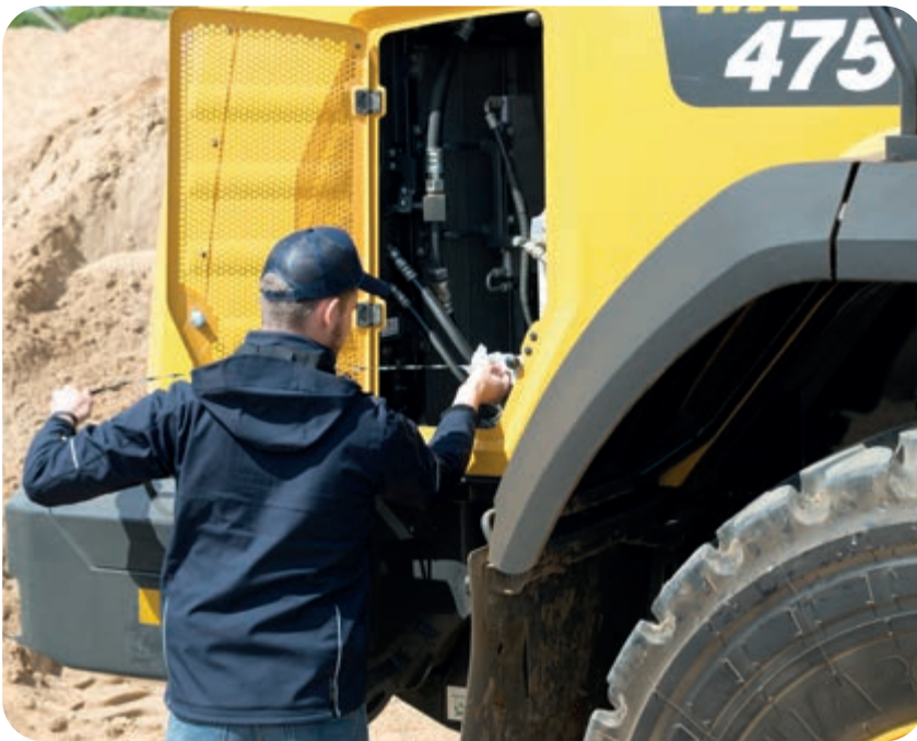
Well located service doors allow convenient and safe access to daily service points
