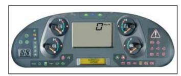
tem not only has an error memory and a self-diagnosis function, but also a service interval display. This significantly simplifies service work and the operator is notified on time of the regular oil and filter changes. The operator and customer-service engineer are constantly informed about the optimum machine state so that problems don't even occur in the first place.
