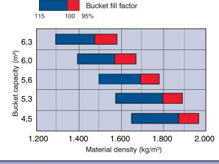
Stock pile bucket Loading loosened material
